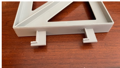
Figure 4: Tabs Glued to Support Truss
