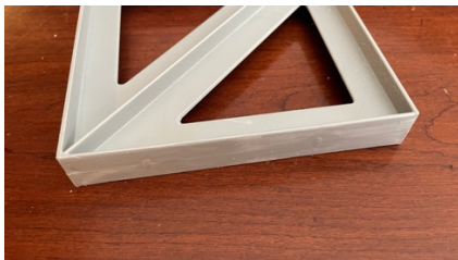
Figure 3: Broken Tabs Removed
